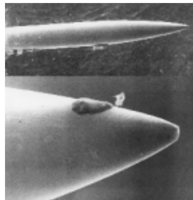
Plate 1 Low (x39.4) and high (x612.5) power magnification of a single needle. The lump on the upper surface of the high power photo can be seen close to the tip on the low power.
