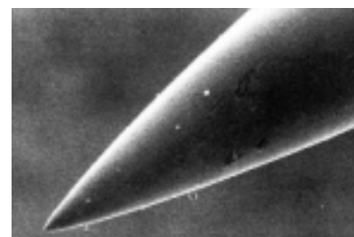
Plate 10 An almost perfect needle-tip (x612.5).
