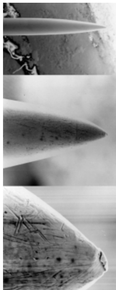
Plate 2 Three magnifications of a single needle (x65, x850 and x5000).
