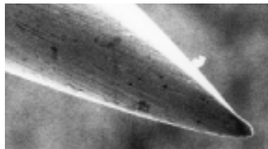
Plate 4 Scratch marks along a needle (x612.5).
