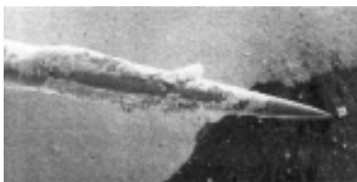
Plate 11 Silicone coating (damaged during microscopy) (x39.4).
